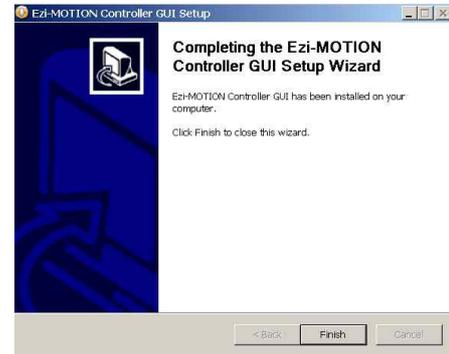
Then installation is completed at the selected folder, 'Program Files/FASTECH/EziMOTION PlusR' folder is created and also GUI icon and program folders are installed.
