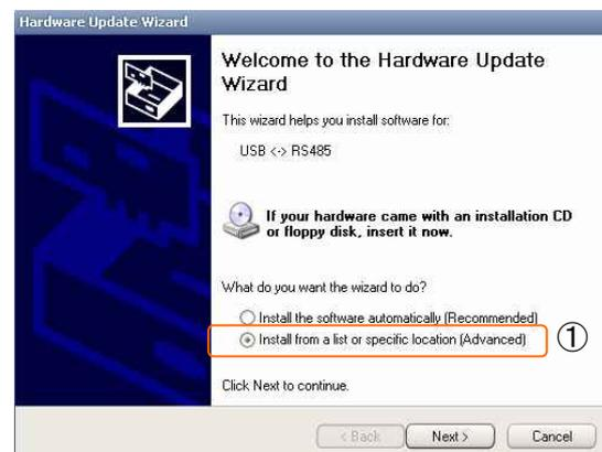
After select the 'FTDI USB Driver' folder (that is installed together with User Program (GUI), click 'Next' button.
